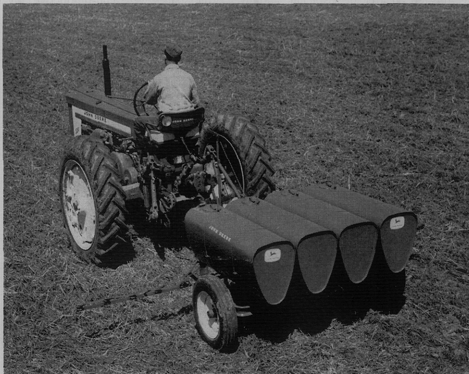
Figure 1: Equipment used to broadcast liquid heptachlor-fertilizer mixture and disk it into the soil for control of soil insects over several seasons
